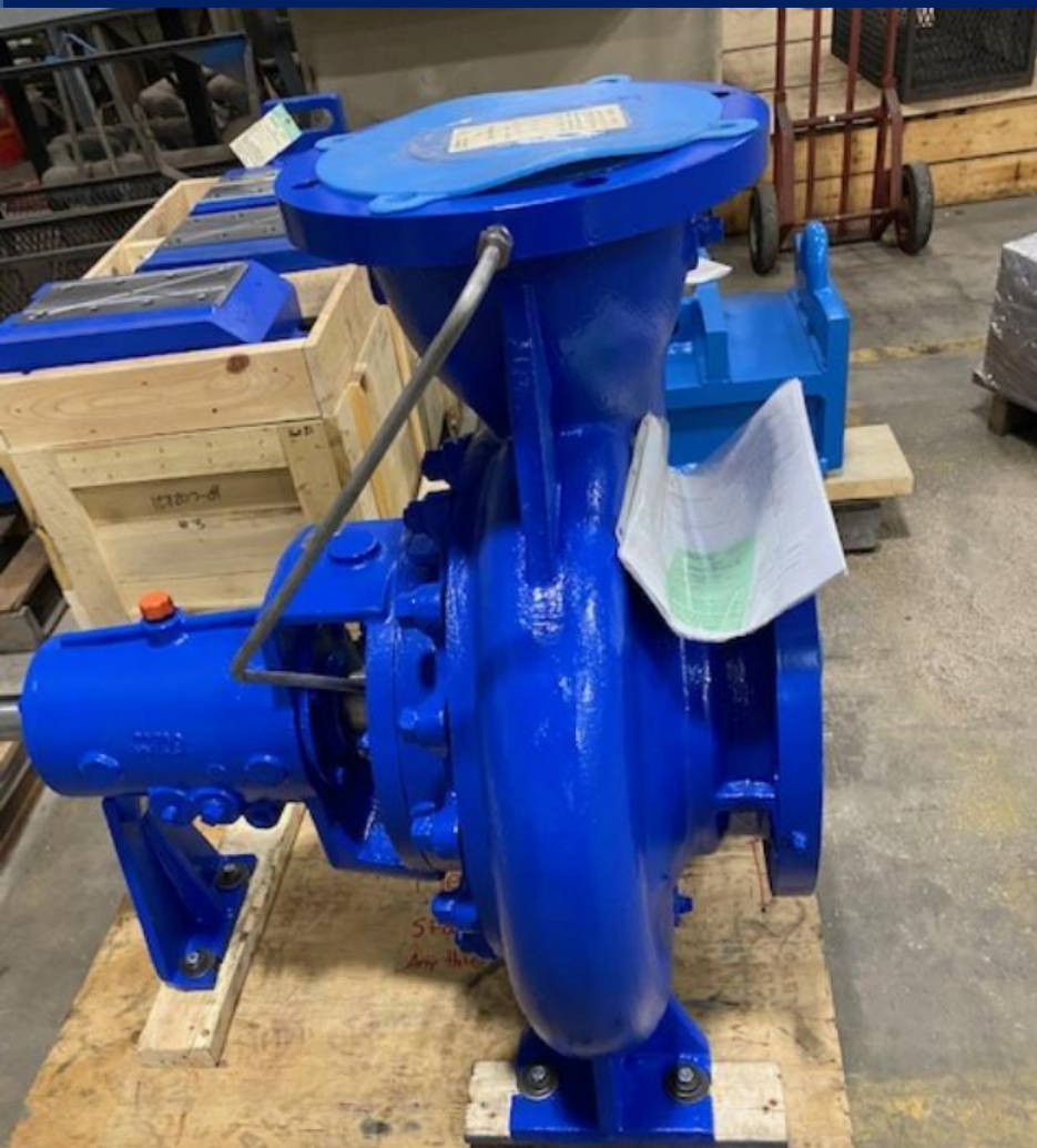
Volute pump Rebuild
