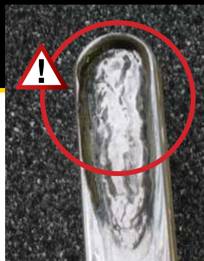
Dangerously eroded gage glass. Eroded glass is often not visible without inspection of disassembled gage.
