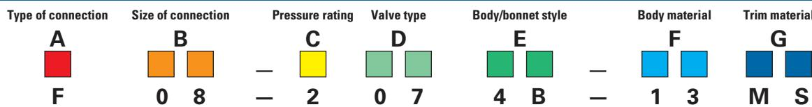
Example: is a NPS 2 (DN 50) 600 Class stainless steel bolted bonnet globe valve with MS trim.
