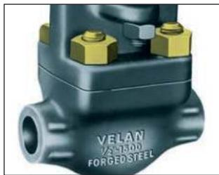
Our bolted joints are calculated to a minimum gasket stress of 16,000 psi which is essential for a leakproof joint. Our fugitive emissions qualification test demonstrated less than 20 ppm performance from gasket joints.
