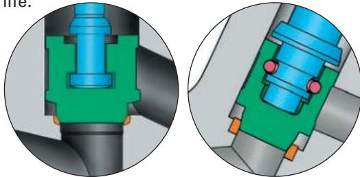
Solid CoCr alloy disc for full CoCr alloy trim
