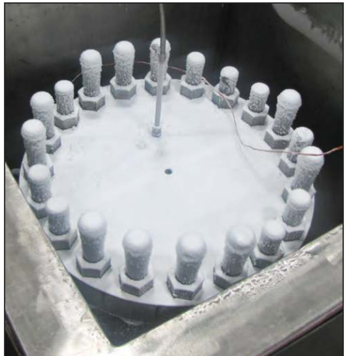
Dual-plate check valve after cryogenic testing.
