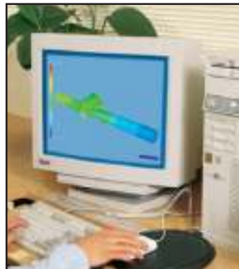
Velan used Computational Fluid Dynamics to improve the flow characteristics of this 4" (100 mm) globe valve.
