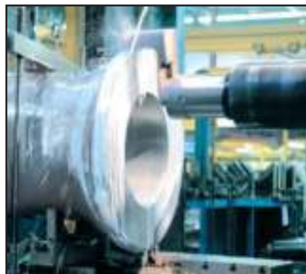
A large CNC horizontal boring mill (with tool changers) machining forged pressure seal bodies.
