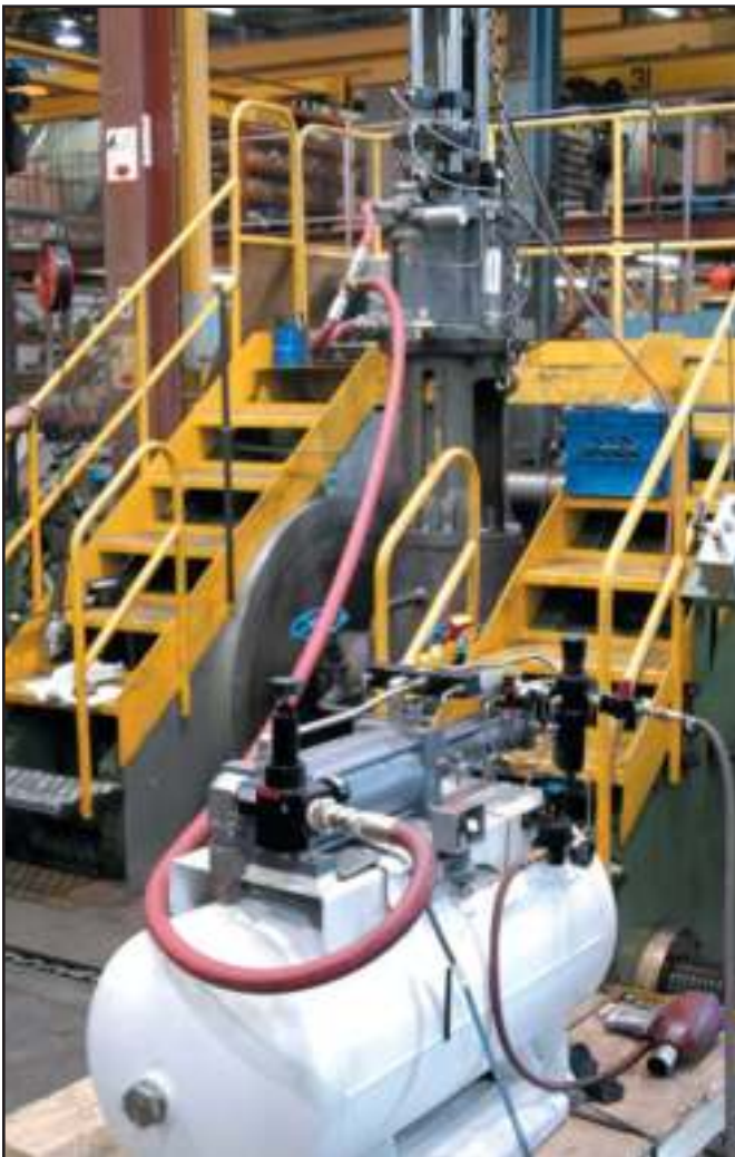
Velan used Computational Fluid Dynamics to improve the flow characteristics of this 4" (100 mm) globe valve.
