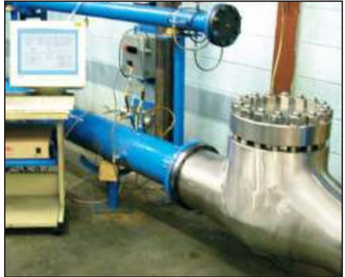
Flow testing on a 10" (250 mm) Class 1500 forged bolted cover swing check valve.
