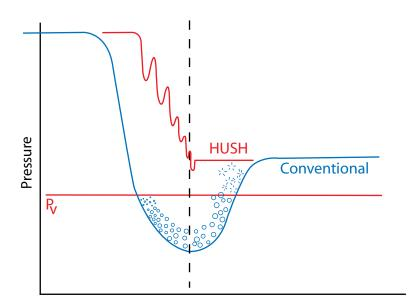
Conventional trim allows damaging cavitation to occur when the pressure drops below the vapor pressure of the liquid. HUSH Trim is designed so that the pressure at the last stage of drop is not at or below the vapor pressure. Cavitation therefore cannot occur.
