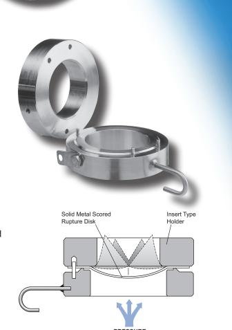
SRA Series Disks mount with the convex surface facing the process media. As pressure increases above the recommended operating ratio, the compressive stress in the disk material increases until a point of instability is reached. At that point the disk begins to buckle. It tears along the score lines as it reverses, which initiates the complete rupture of the disk.
