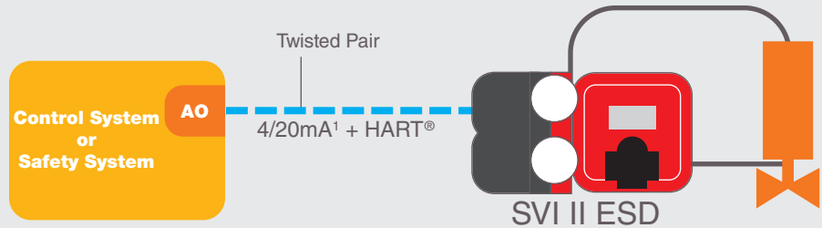
2-wire solution – Safety function triggered by current sensing (i.e. 4mA = Safety Trip)
