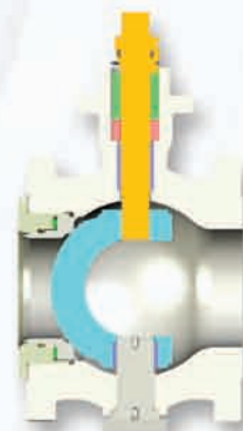
Heavy Duty Seat option provides increased durability in harsh services.
