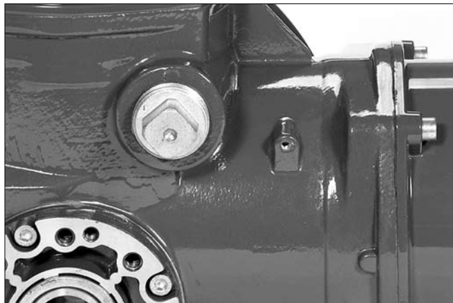
Figure 3.20 – External earth/ground connection – housing
