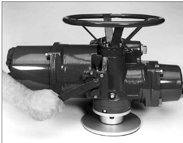
Figure 3.23 – Declutch lever shows direction of engagement (MX-05 shown)
