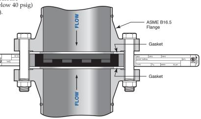
If company policy or jurisdictional regulation requires ASME Code compliance, the rupture disk devices used for pressure vessel overpressure protection shall bear the ASME Code UD symbol. The UD marking is the manufacturer's declaration that the device was manufactured in full compliance with the ASME Code.
