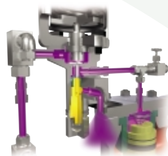
PV Valve Open (Relieving Position)
